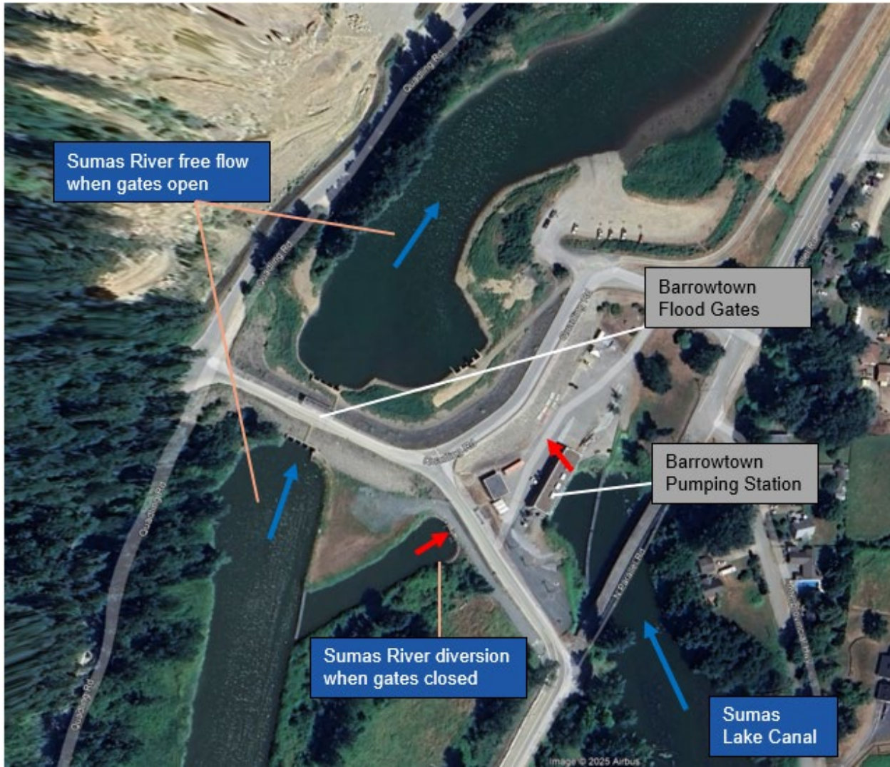
Figure 2.4 Barrowtown Pump Station Complex Schematic
